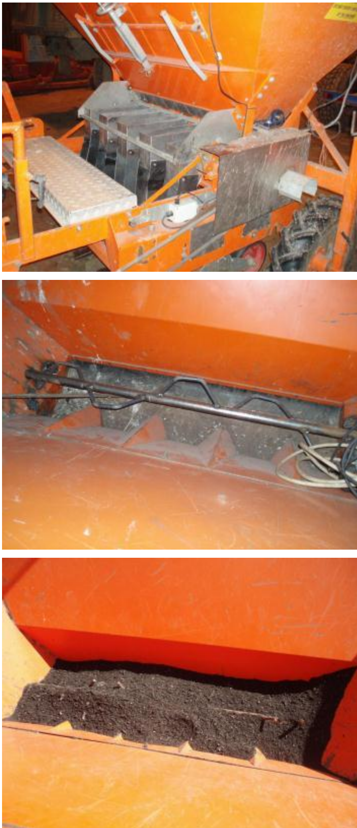
Fig. 1. Converted set planter for applying compost along the planting row.
